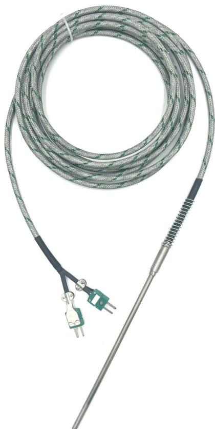
TERMOPAR TIPO K DOBLE INCONEL 600 AISLADO DE MASA ENTRE SI, Ø6MM, L200MM CON 5000MM DE CABLE 4X0,8MM,SILICONA-FIBRA-MALLA.
