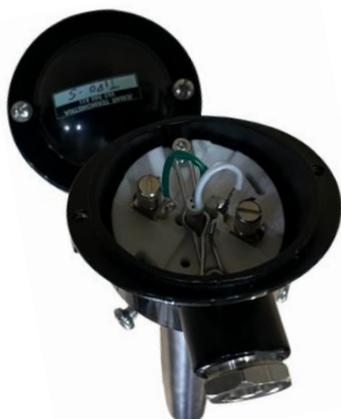
TERMOPAR TIPO S Ø27MM L2012MM, HILO Ø0,5MM, CABEZA DIN-A, VAINAS CERAMICAS C530 Y C610 DE 2030MM, CASQUILLO INOX Ø33X300MM
