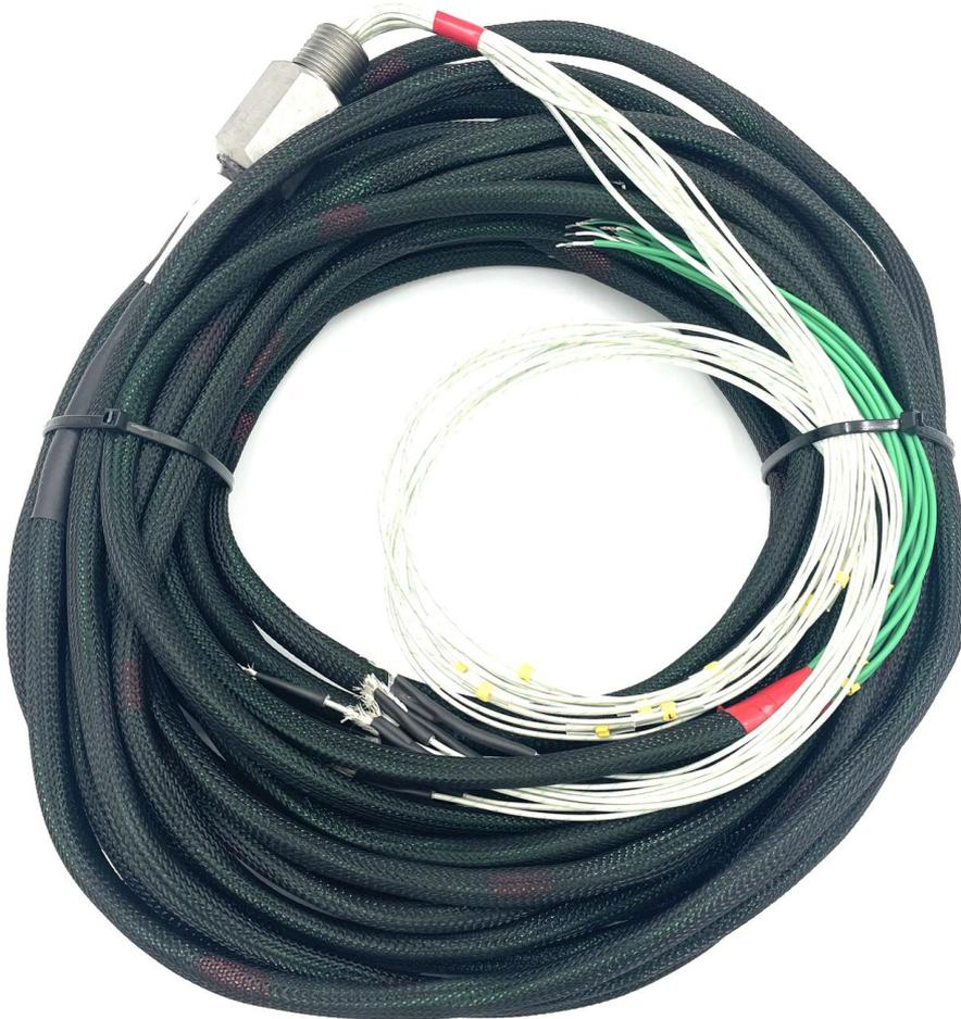
ALARGADERA TERMOPAR TIPO J, 10 CANALES, 3/4" 1MTS TEFLON INTERIOR 20MTS PVC EXTERIOR
